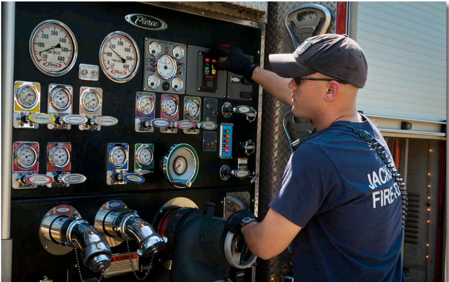
Engine 1’s Eng. Billy Green monitors and adjusts water pressure during a relay pumping cluster drill on April 2.
